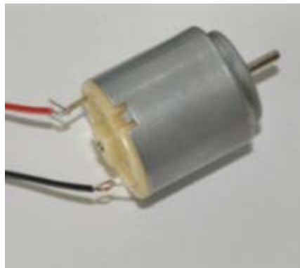
Figure: motor with wires on contact poles.
