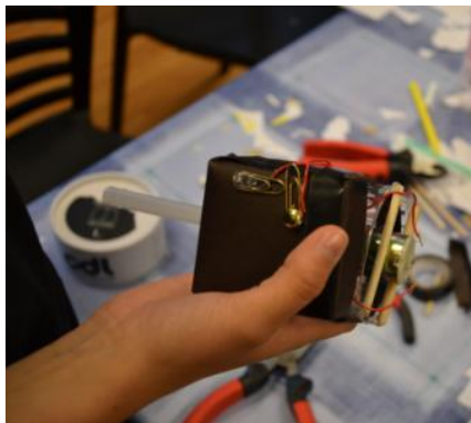
Figure: vacuum cleaner with a switch.
