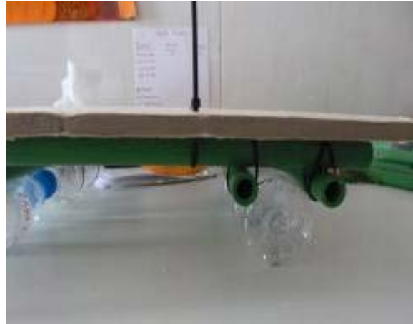
Figure 9. Fastened mountboard on the frame of the platform.
