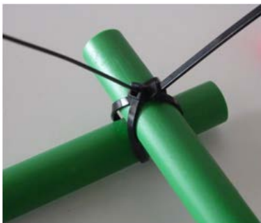
Figure 1. Zip ties used to tie the PVC pipes together. In the figure you can see that the zip ties are crossed. In that way you can make sure that the bond will be strong enough.
